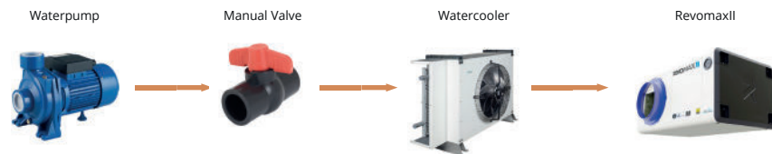
Manual valve install sequence
